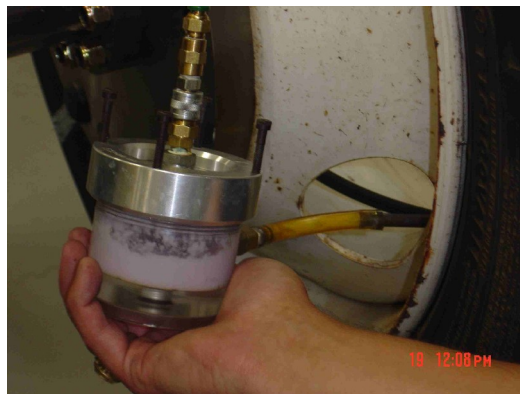
Installation of Ride-On Brand Sealant via a Pressure Pot
